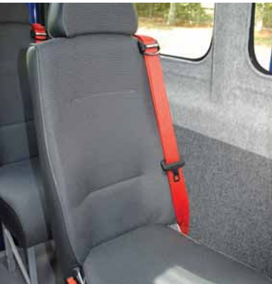
All-age 3 point seatbelts and seatbelt anchorages tested to EEC Directive
