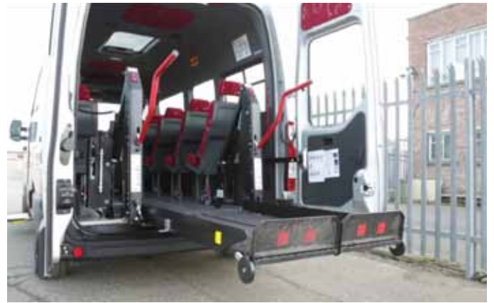
On board split platform lift for convenience and ease of wheelchair loading.
