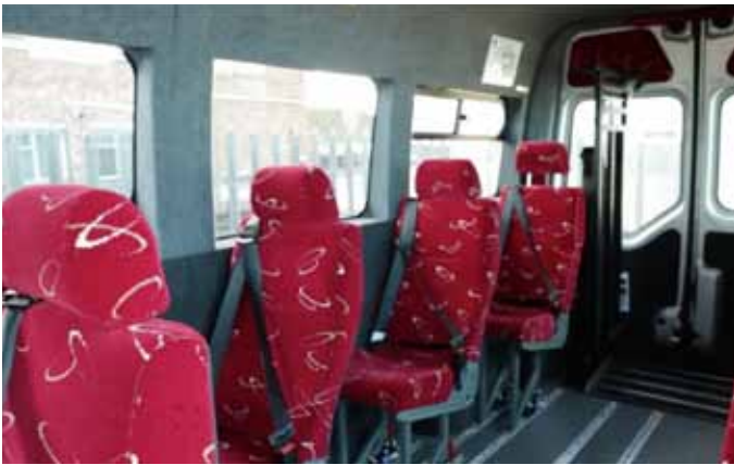
Fully tracked tested floor complete with fully removable seating.
