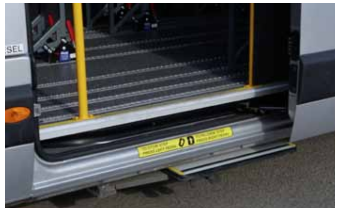
Manual side step for low entry and ease of boarding.
