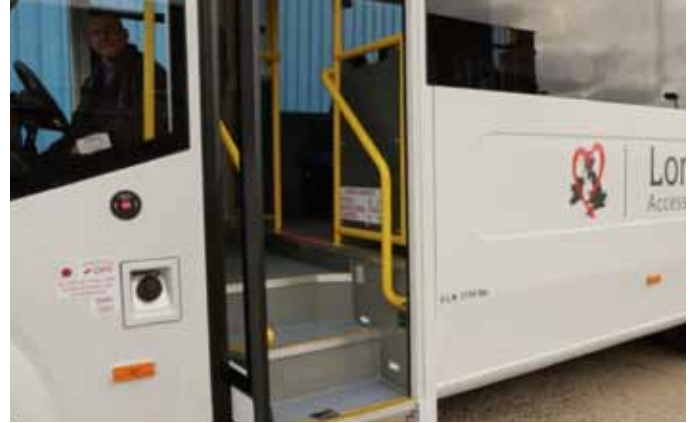
LED entry step lighting.
