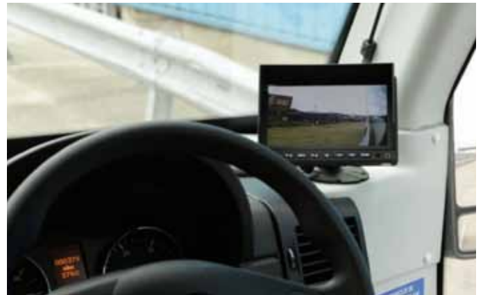
Reversing and side mounted cameras with dashboard screen display and proximiter alarm.
