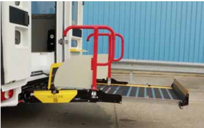
PLS access underfloor lift 1410mm x 825mm 400kg load capacity as standard.
