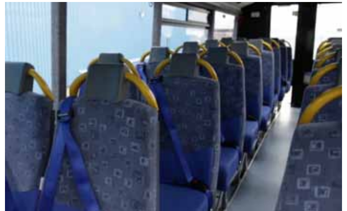
Open style grab handled headrest designed to assist and support the passenger.
